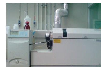
IC coupled to ICP-MS
